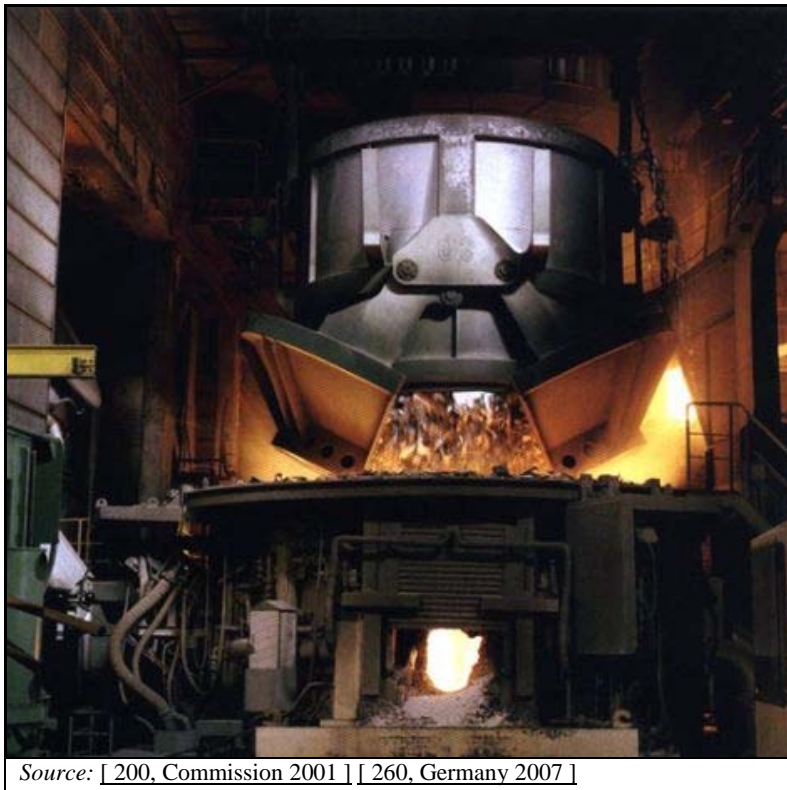
Figure 8.2: Electric arc furnace charging
