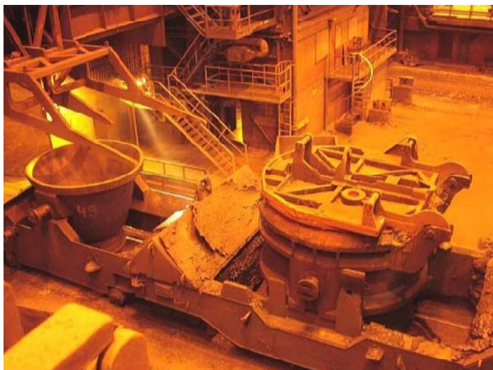
Figure 7.24: Automatic ladle lid system
