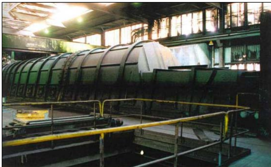
Figure 3.21: Covered sinter strand according to the EOS process
