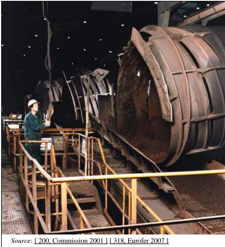
Figure 4.1: Balling drum as part of a pelletisation plant where the green pellets are formed
