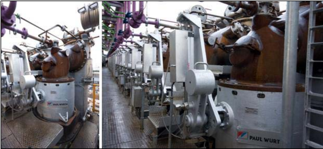
Figure 11.5: SOPRECO Model 2 valves on a stamped charged battery
